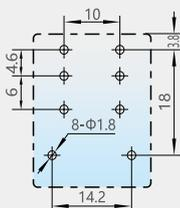
PCB安装孔位图(2ZS)
